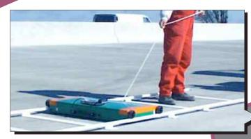
MIT-DOWEL-SCAN. We proudly introduce MIT-DOWEL-SCAN the latest development in Non-Destructive determination of dowel and tie bar positions in plain concrete. The MIT-DOWEL-SCAN is a totally new device allowing the operator to measure and evaluate pavement joints in real-time without using a rail system. The device makes use of the magnetic properties of the dowel bar by recording its returned magnetic field via sensors.
