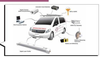
Network Survey Vehicle for complete road analysis and Road condition and Pavement analysis in defining true condition of road network. Network Survey Vehicle (NSV) mounted with equipment for Row and surface pavement defects, high accuracy DGPS receiver and in vehicle data processing so ware to accurately measure pavement surface properties such as cracking, potholes, raveling, rutting and roughness.
