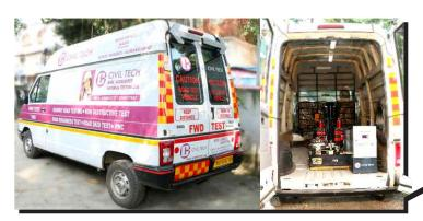
FWD is a vehicle mounted device which helps in distributing the load evenly. It's being used for NDT and evaluation of load carrying capability of highways, pavements and airfields. Data collected from FWD can be used for determination of structural capacity of in-service pavements/Roads for analytical analysis of their performance. Analyses of data are being carried out using standard so ware as supplied by the manufacturer.
